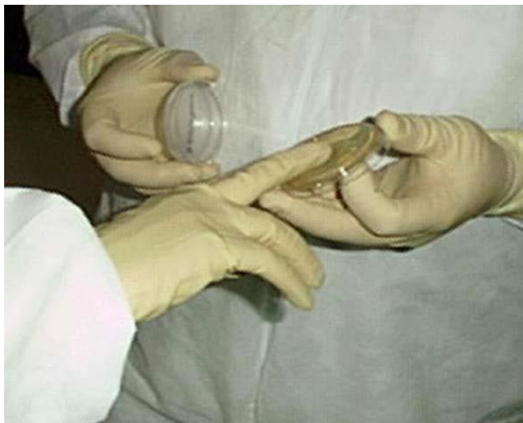
Figure 8-14. Microbial personnel testing: gloved fingertip RODAC testing
