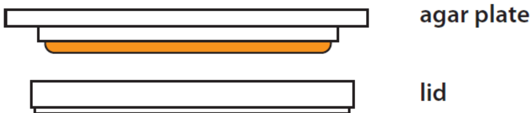
Figure 8-12. RODAC plate is a contact impression plate used for microbial monitoring of surfaces
